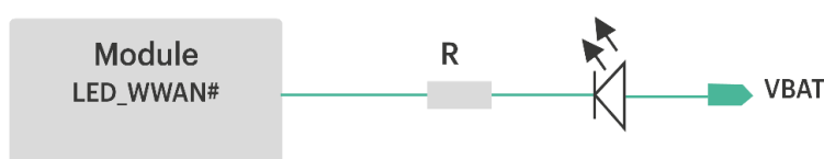
Figure 5 Circuit diagram of network indicator
