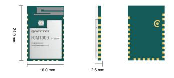
FCM100D is a cutting-edge MCU Wi-Fi and Bluetooth module launched by Quectel. It boasts a high-performance processor with a frequency of up to 120 MHz and supports IEEE 802.11b/g/n protocol and BLE 5.2. The module features built-in 256 KB RAM and 2 MB/4 MB flash, ensuring efficient performance. In addition, it complies with WPA-PSK, WPA2-PSK and WPA3-SAE security standards.
