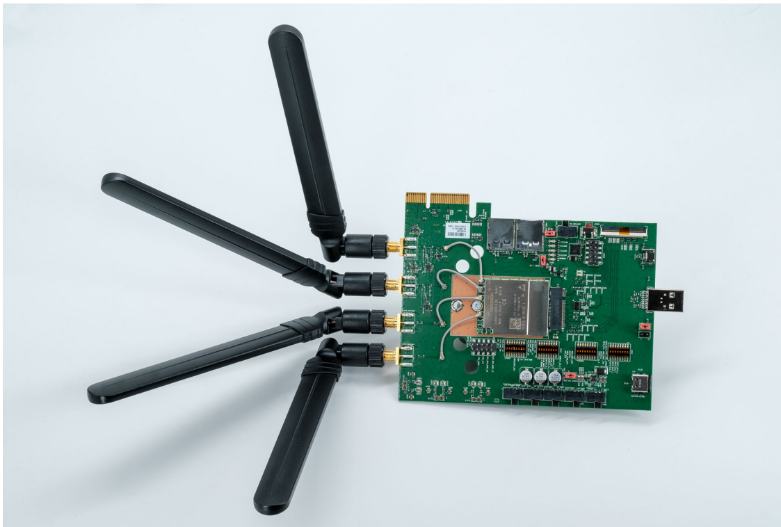
Figure 2: MV31-W mounted on 5G Modem Card Adapter Board
