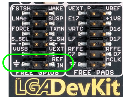
Figure 12: External reference supply and pin header for free level shifter
